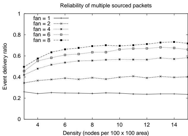
Fig. 3. **Multiple sourced packets:** This illustrates the ratio of events received with respect to density. For one sourced packet, the ratio is extremely low; however the reception dramatically increases with additional sourced packets for each event.
