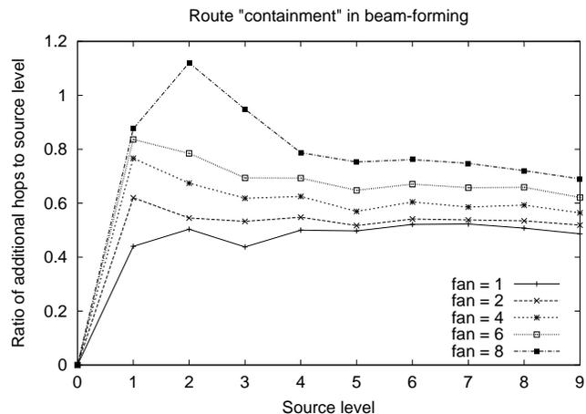
Fig. 6. **Route “containment”:** This shows the relative number of additional hops (actual route length - shortest route length) packets take while traveling from a source to the sink for various fanouts. The metric measured is the ratio of the additional hops to the level of the source.
