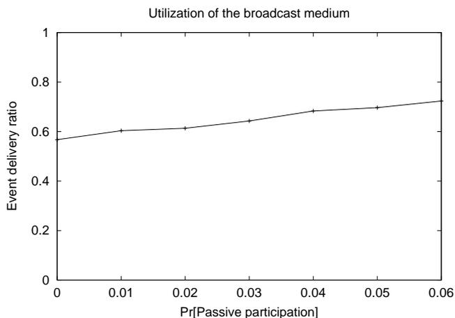
Fig. 5. **Passive participation:** Utilizing the broadcast medium, this figure shows the improvement in event reception over various probabilities of participating in passive packet processing. These results were recorded for four sourced packets on graphs of density equal to ten.
