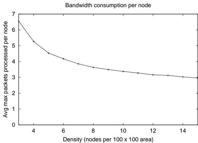
Fig. 4. **Bandwidth:** For eight sourced packets per event, this figure depicts the bandwidth consumption. One event occurs per simulation and the maximum number of packets processed by any given node for the entire simulation is recorded. The results of a series of simulations are averaged.
