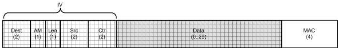
(a) TinySec-AE packet format
