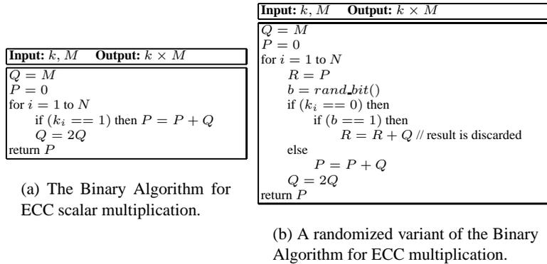
**Fig. 1. Introducing randomness into the Binary Algorithm for ECC scalar multiplication.**
